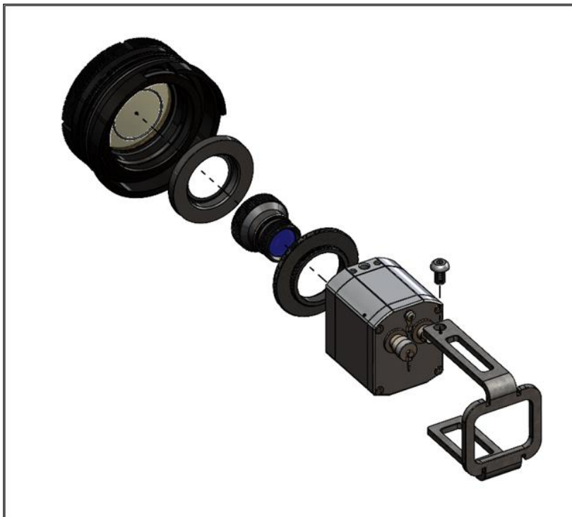
Figure 19: Assembling of the 80° optics
