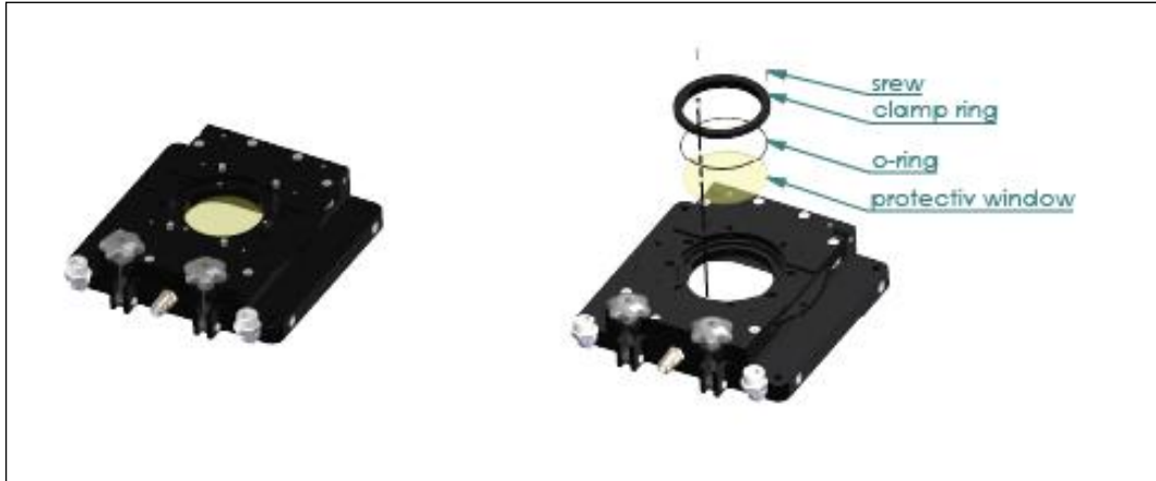
Figure 54: Change of the protective window
